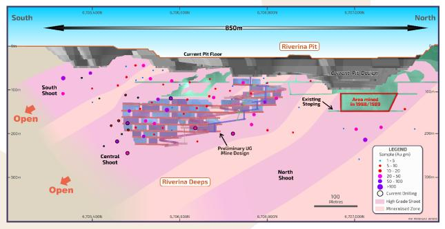
Figure 2 -Long Section A - A' showing high grade shoots and area of recent underground mining
